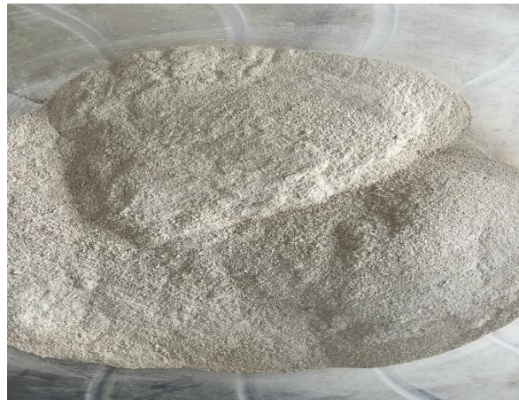
Plate 3.3 Eggshell powder after mechanical grinding.
