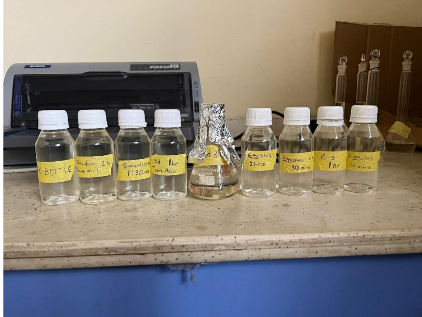
Plate 3.12 Digested produced water samples prepared for analysis via Atomic Absorption Spectrophotometry (AAS)
