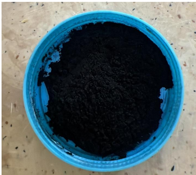
Plate 3.10 Fully activated sawdust adsorbent after the complete thermal and chemical treatment process.
