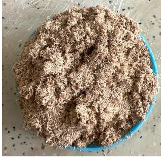
Plate 3.6 Sawdust after initial mechanical grinding.
