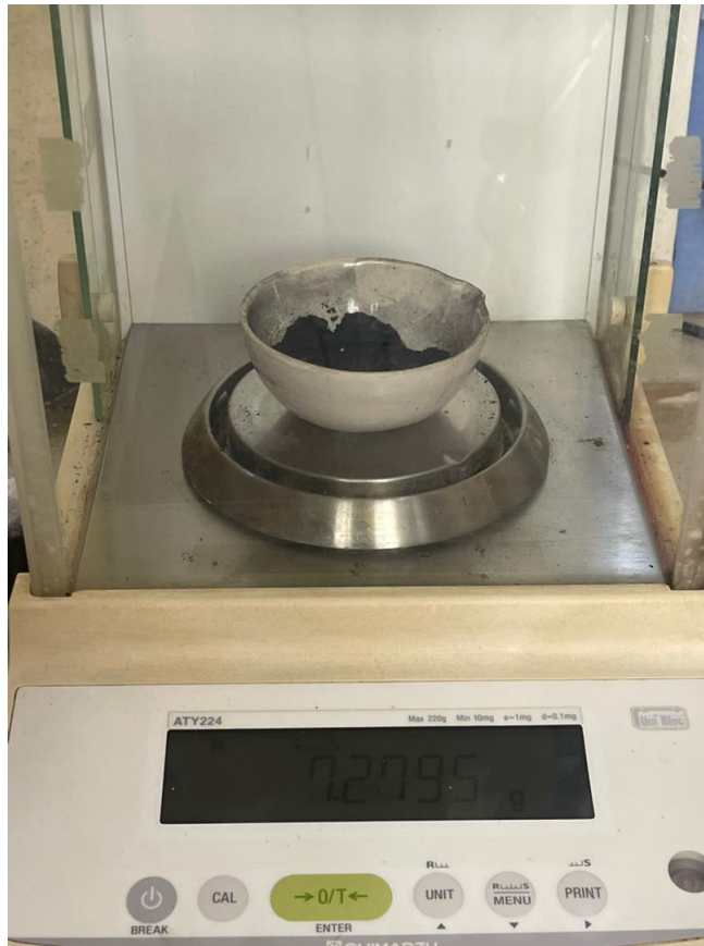
Plate 3.9 Mass measurement of the 10g sawdust sample after the complete acid activation and drying process.
