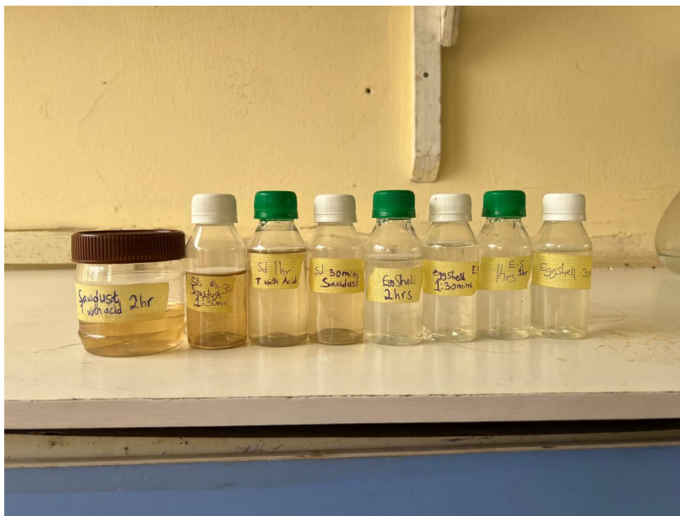
Plate 3.11 Treated produced water samples at different contact times
