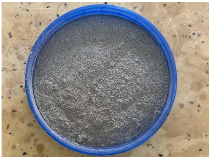
Plate 3.4 Thermally activated eggshell powder after calcination at 700°C and sieving.
