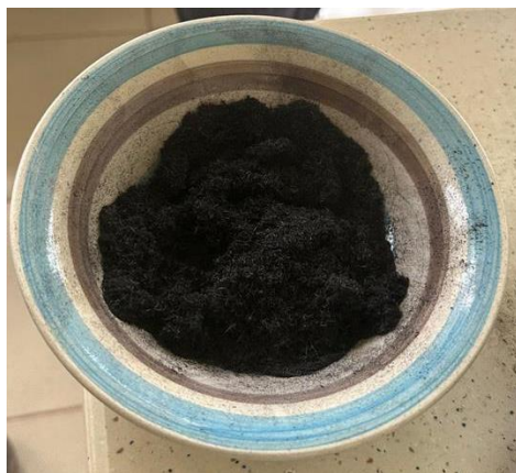
Plate 3.7 Sawdust after thermal activation at 300°C, before final grinding and sieving.
