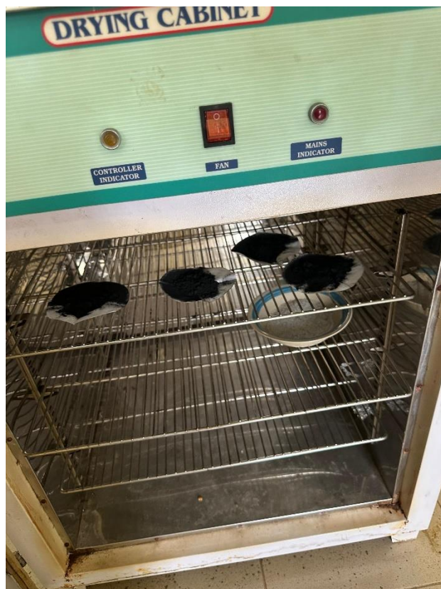
Plate 3.8 Chemically activated sawdust undergoing oven drying after washing to neutrality.
