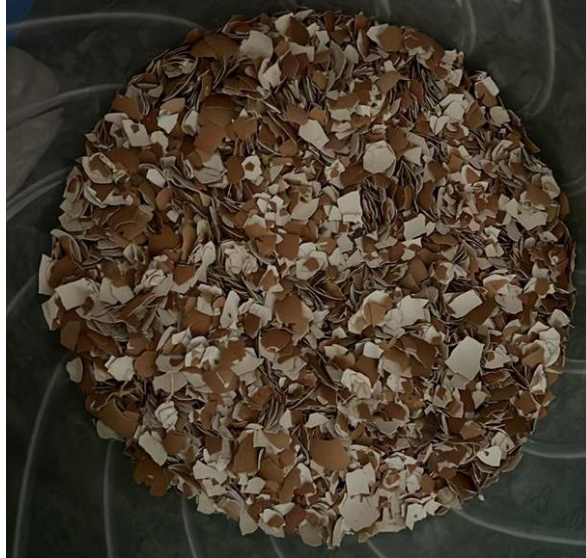
Plate 3.2 Eggshells after membrane removal, rinsing and sun-drying.
