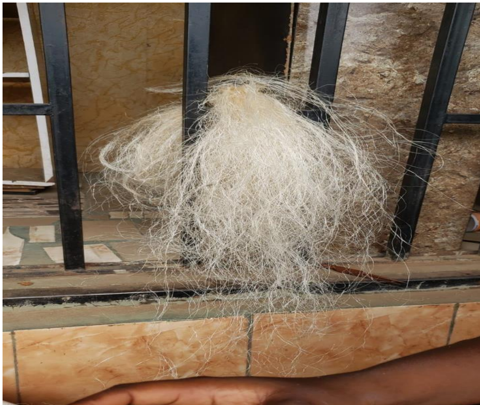
Fig 3.7: Extracting plantain fibres
