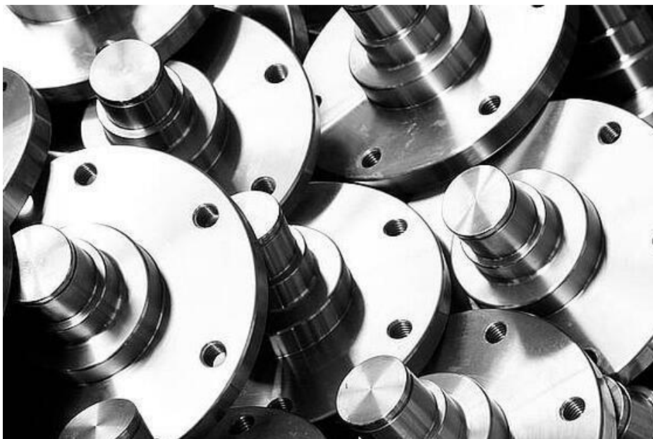
Figure 2.1 Machine application of C45/AISI 1045 steel (a medium carbon steel); suitable for part such as gears, bolts, general-purpose axles and shafts, keys and studs. (Source: Weerg, 2021).
