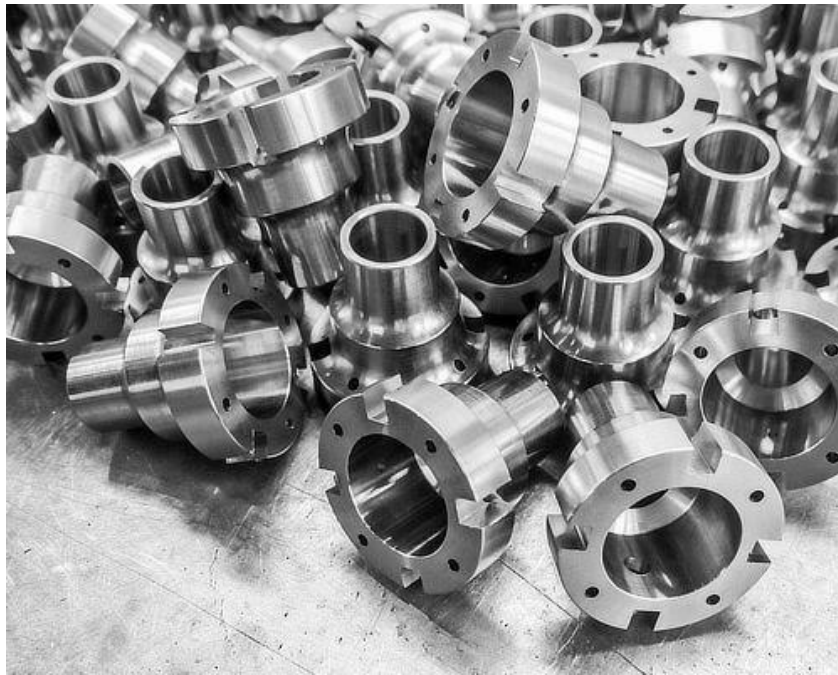
Figure 2.2 Machine application of AISI 4317/18NiCrMo5 alloy steel having high core strength and toughness: used on heavy duty bearings, cam followers, clutch dogs, compressor colts, fan shafts, heavy duty gears, pump shafts
