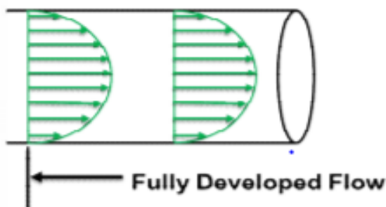
Fig.2. 6 Velocity Profile of Developed Laminar Flow
