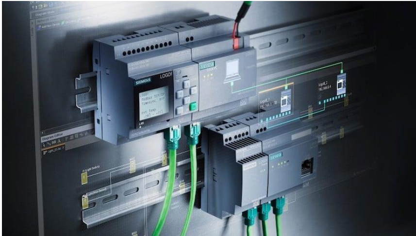
Figure 9- a programmable logic controller
