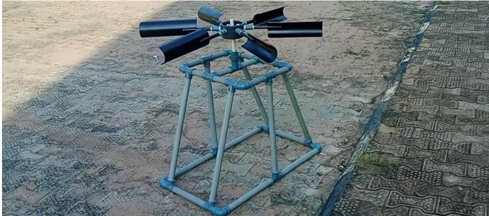
Figure 4.1: Photograph of the assembled 500W wind turbine
