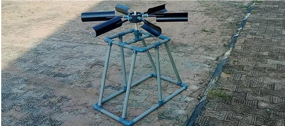
Figure 4.1: Photograph of the assembled 500W wind turbine
