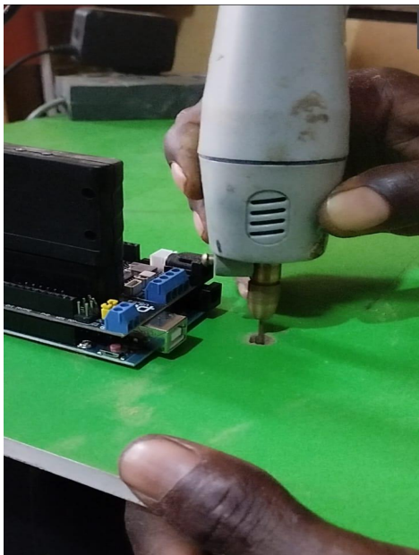
Figure 4.14 – Image of hole being drilled on the wooden board
