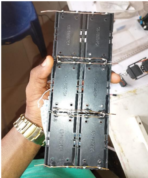
Figure 4.12 – Image of Battery holder soldering
