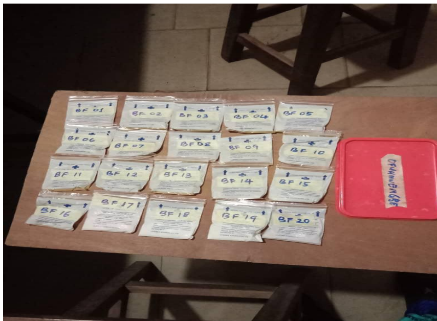
Figure 3.6. Ofunmwengbe samples ready for XRF analysis.
