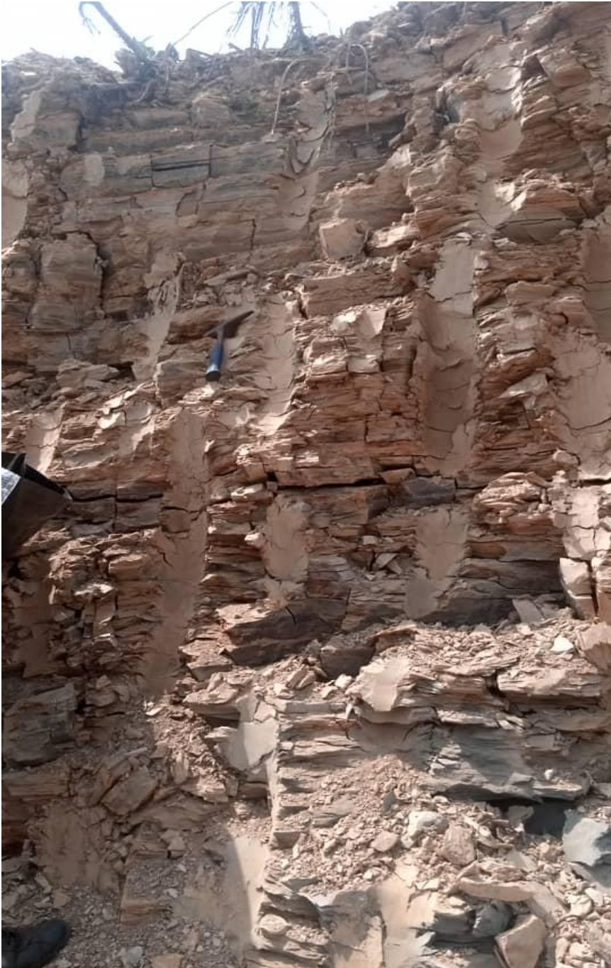
Figure 2.3a. Clay deposits with interbedded layers of shale and clayey shale layers at Ofunmwengbe sample location
