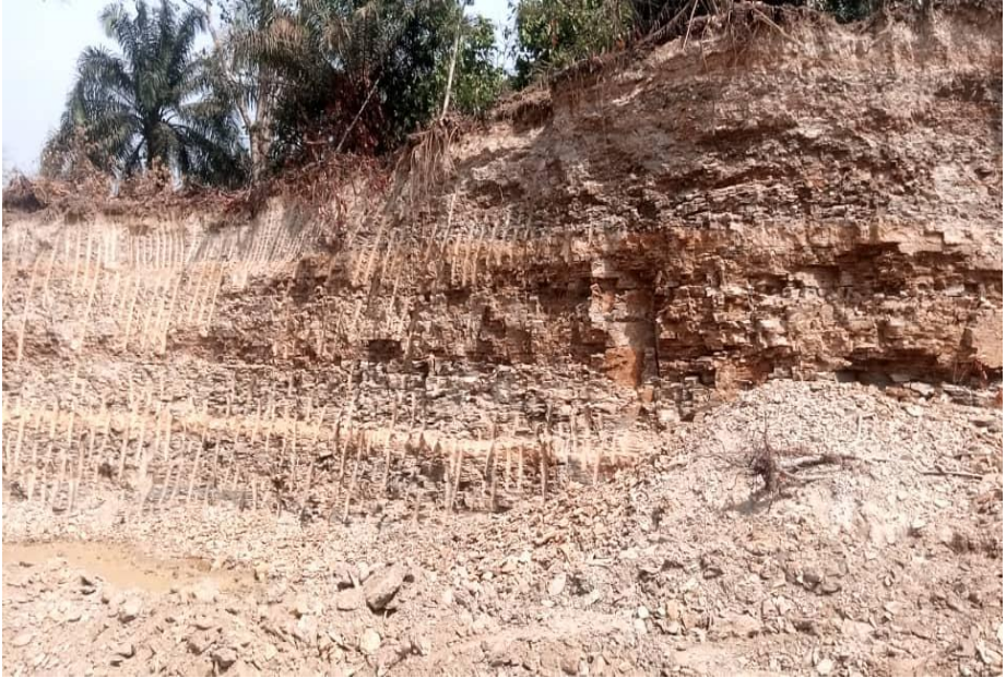
Figure 2.3b. Sedimentary profile of iron cap stones, sandstones with intercalated clay layers at Ofunmwengbe.
