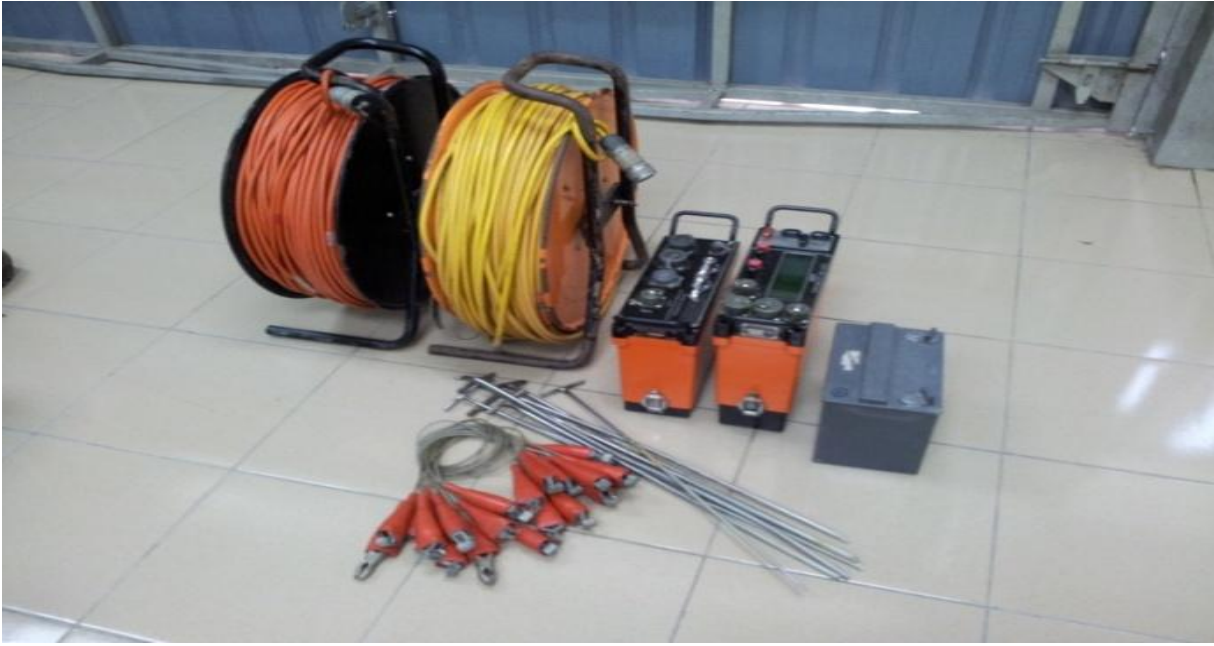
Figure 3 6: Terameter, electrode selector, multicore cables, clips, electrodes and battery.
