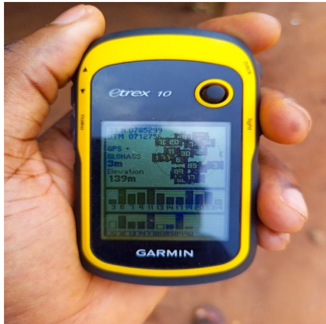
Use of hand held GPS device to obtain co-ordinate of point of collection of sample
