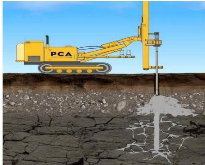
Figure 2.1: Cement Grouting (Shanko, 2017)
