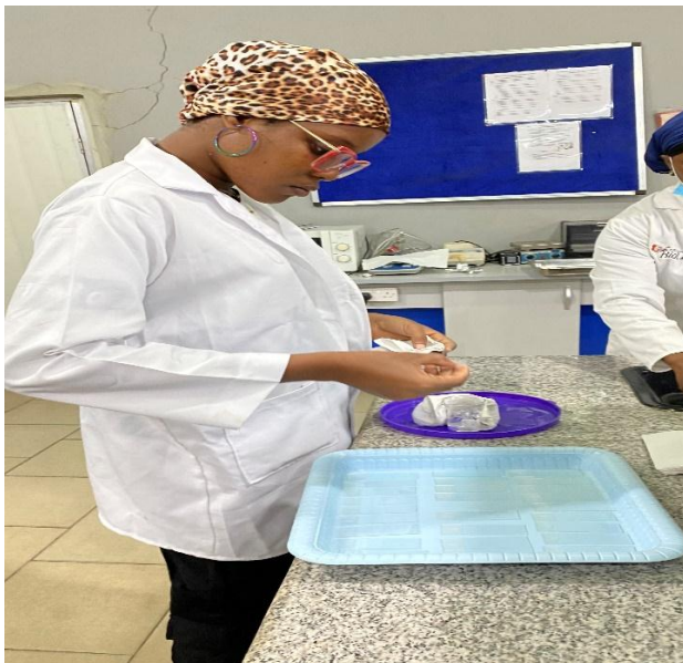
Plate 3.3: embedding slides in normal agarose
