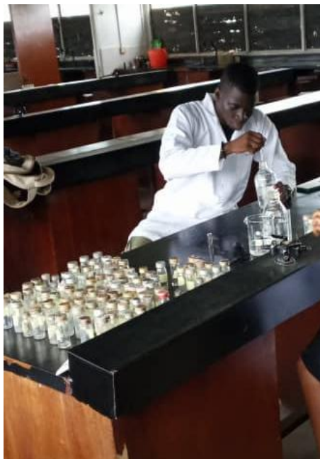
Picture showing Preparation of Quarter-strength Ringer's Solution & dispensing into sterile glass bottles
