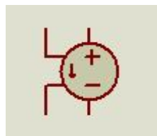
Figure 3.7: Current Controlled Voltage Source
