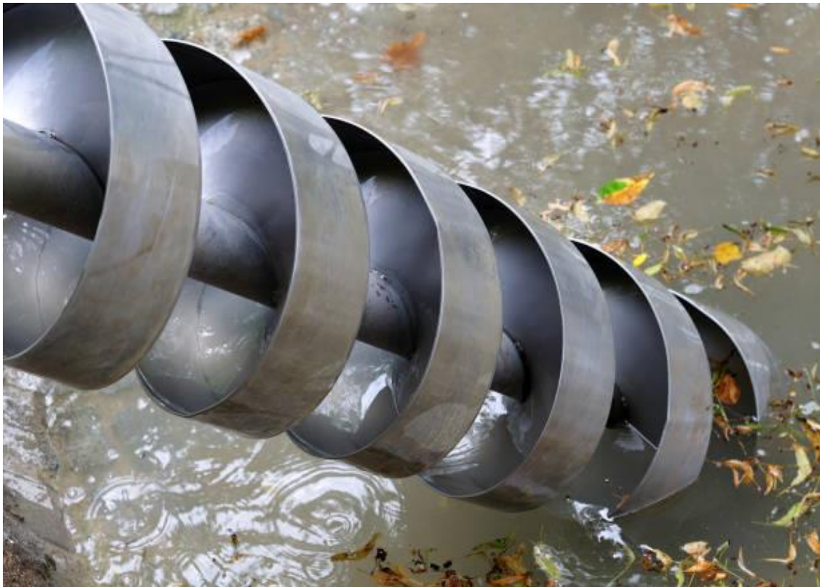
Figure 2.3: The Archimedean Screw Pump
