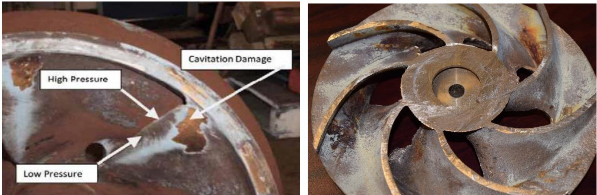
Figure 4.14: Impeller images showing cavitation areas during maintenance
