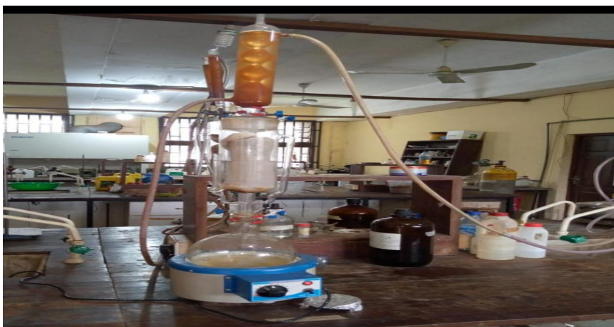
Plate 1: A Soxhlet Extractor (Picture Courtesy: Chemistry Annex Lab, 2022)
