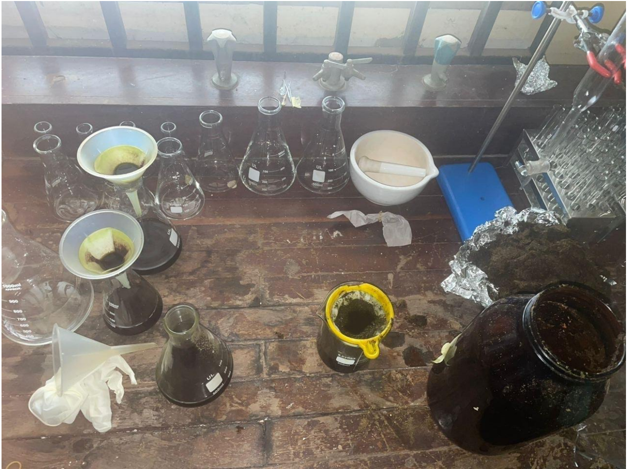
Filtration (after 72 hours of maceration) using Whatman Grade 1 filter paper.
