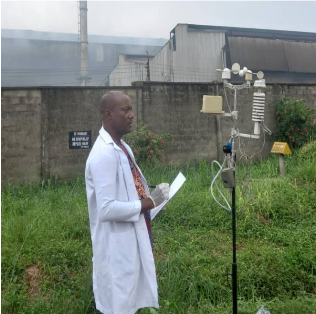
Plate 3: Apex2Is Standard Pump Fitted to Conical Inhalable sampler supported with Professional weather station equipment
