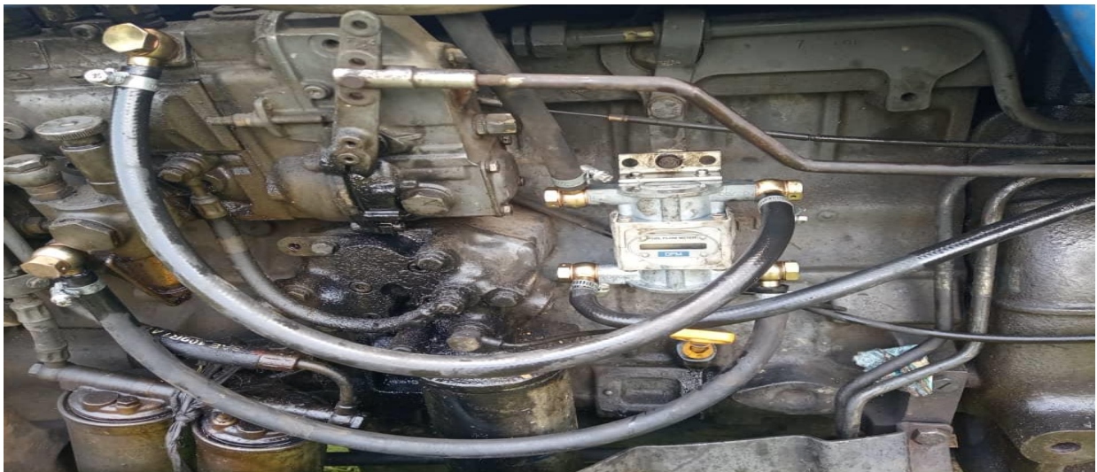
Plate 3.10: Mounting of Fuel Flow Meter
