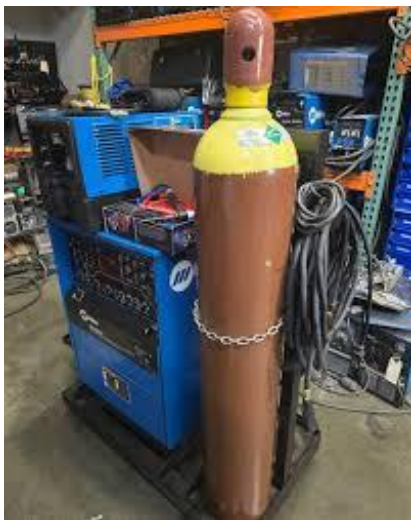
Fig 1: TIG welding equipment with argon gas cylinder
