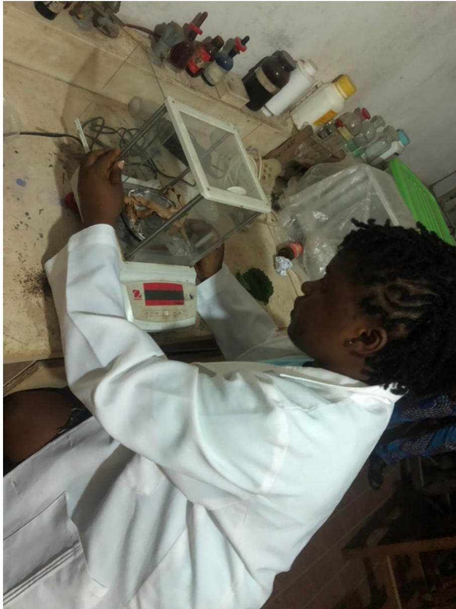
Plate 3: Taking fresh and dry weight measurements of Eichhornia crassipes
