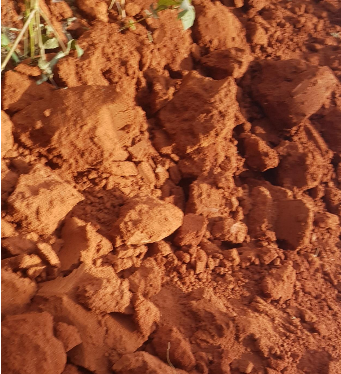
Plate 3.4: Soil samples from profile pit of Idunowina area, showing soil lumps, clayey nature and colour. Source: Author's Field Work 2023
