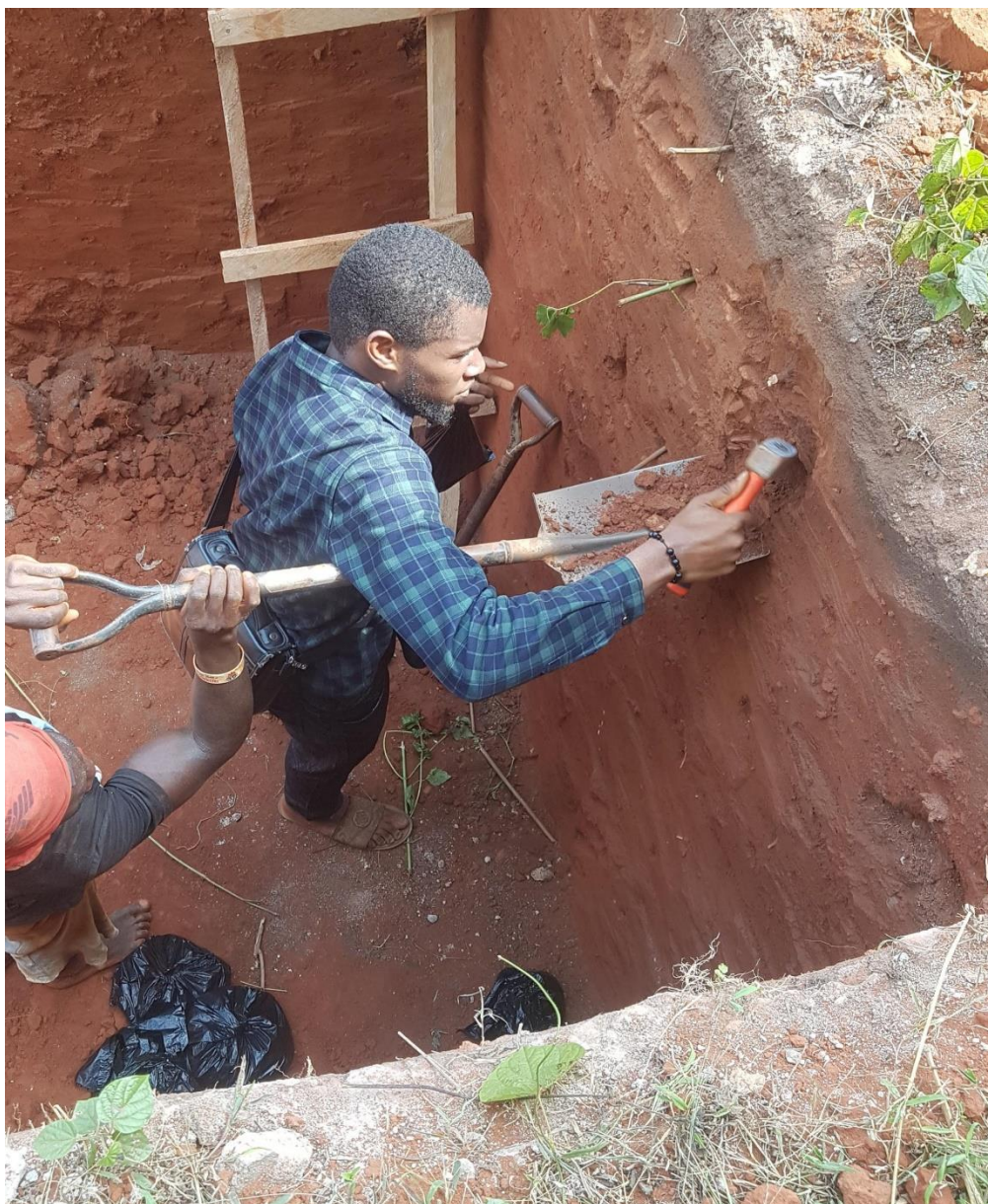
Plate 3.1: Collection of Soil Samples from Profile Pit of Idunowina Source: Author's fieldwork (2023)
