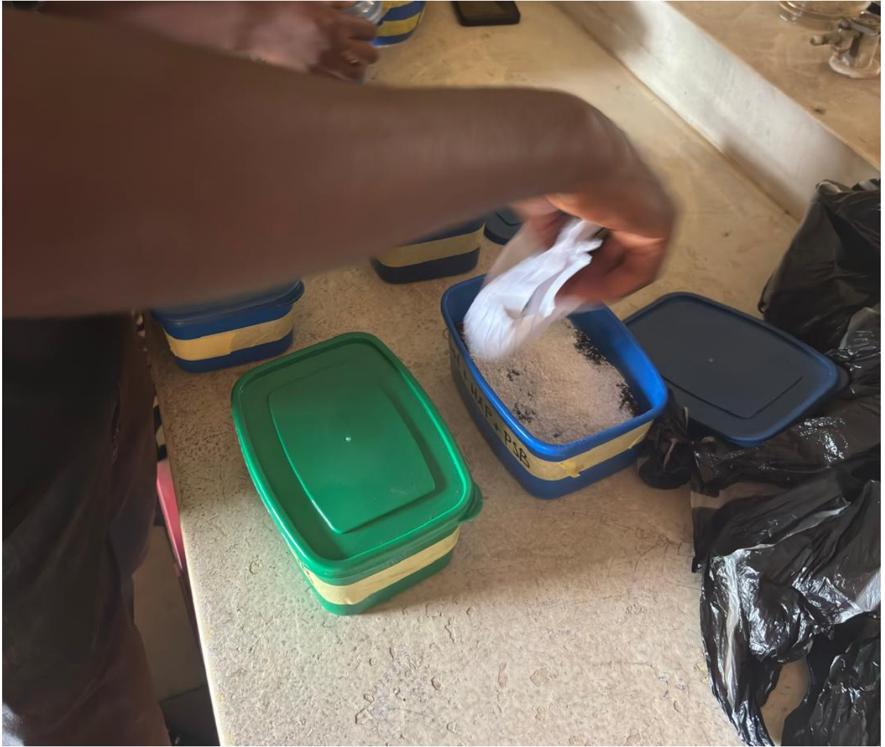
● PLATE 3.5.3.1: Addition of hydroxyapatite to soil samples
