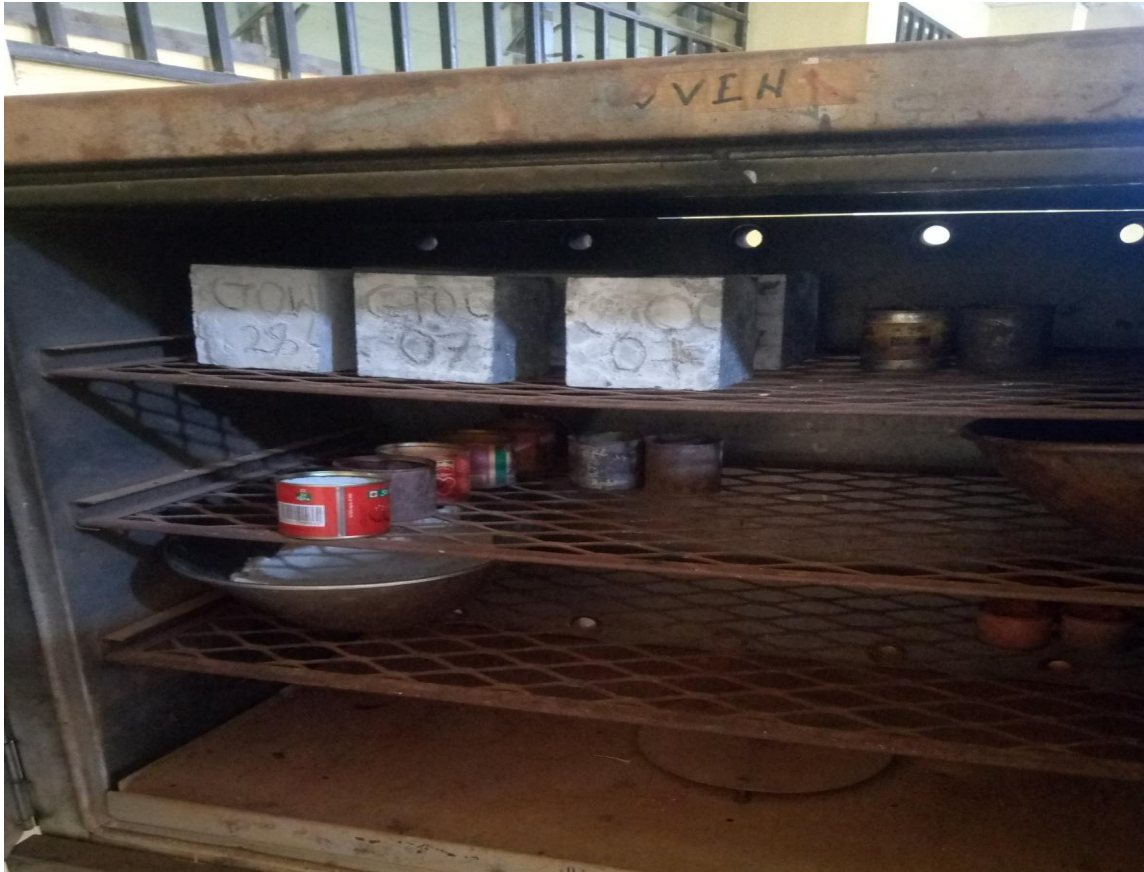
Figure: A- 8: Concrete samples in an oven for water absorption test
