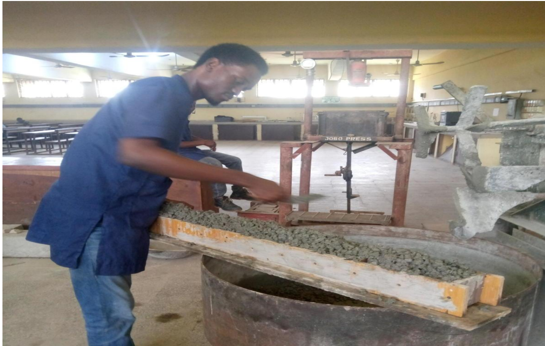
Figure A - 4: Student placing fresh concrete in a mould
