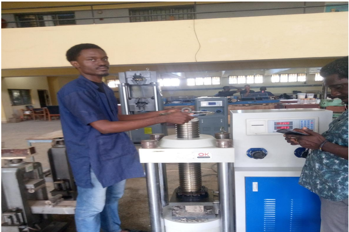
Figure A - 7: Student carrying out compressive strength test on the hardened concrete samples
