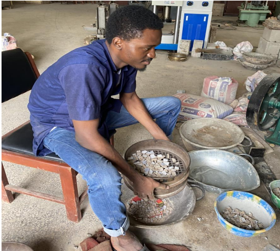
Figure A - 2: Student carrying out sieve analysis of the waste ceramic tiles aggregate
