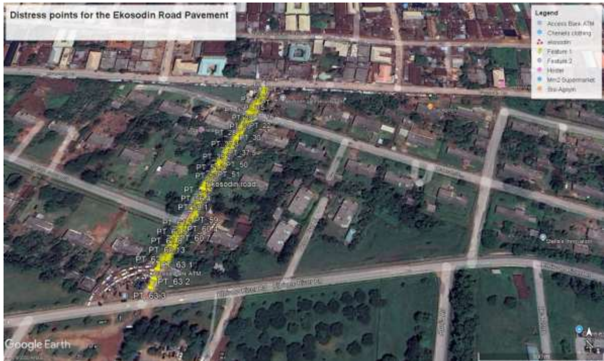
Figure 4.1: Results obtained along Ekosodin Road, University of Benin, Ugbowo Campus, showing the spatial distribution of all distress points in the area (Google Earth).
