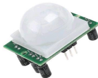
Fig 3.6: PIR Motion Sensor
