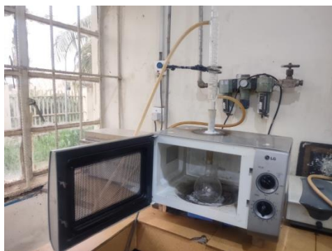
Plate 3.1: wco placed inside the microwave
