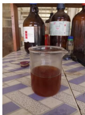
plate 3.4: clean biodiesel obtained after drying
