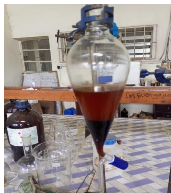
Plate 3.2 separation in the separating funnel
