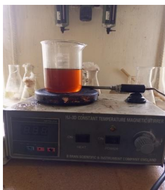
Plate 3.3: drying of biodiesel
