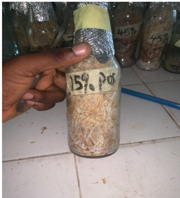
Plate 2: Inoculation of rice straw and palm oil sludge mixture.
