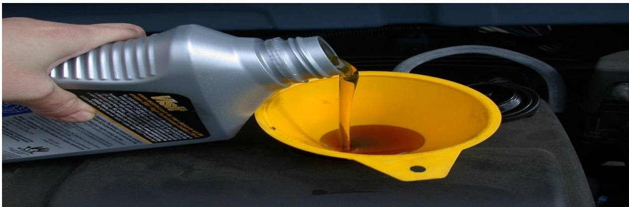
Figure 2.1. Using a funnel to assist with a motor oil refill
