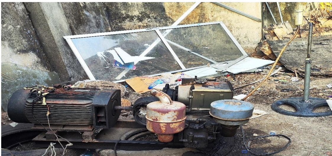
Plate3.6: IC engine and the experimental set-up for combustion of fuels.
