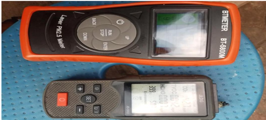
Plate 3.8: BTMETER BT-5800M and JD – 302. (Used for testing for TVOC and CO 2 emission)
