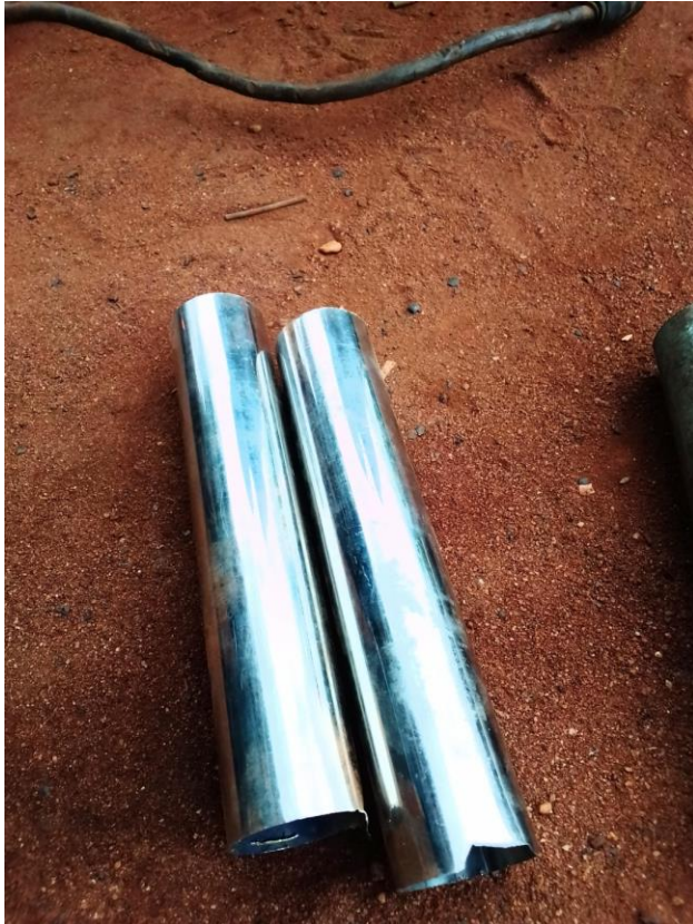
Fig 3.2: Stainless steel pipe.
