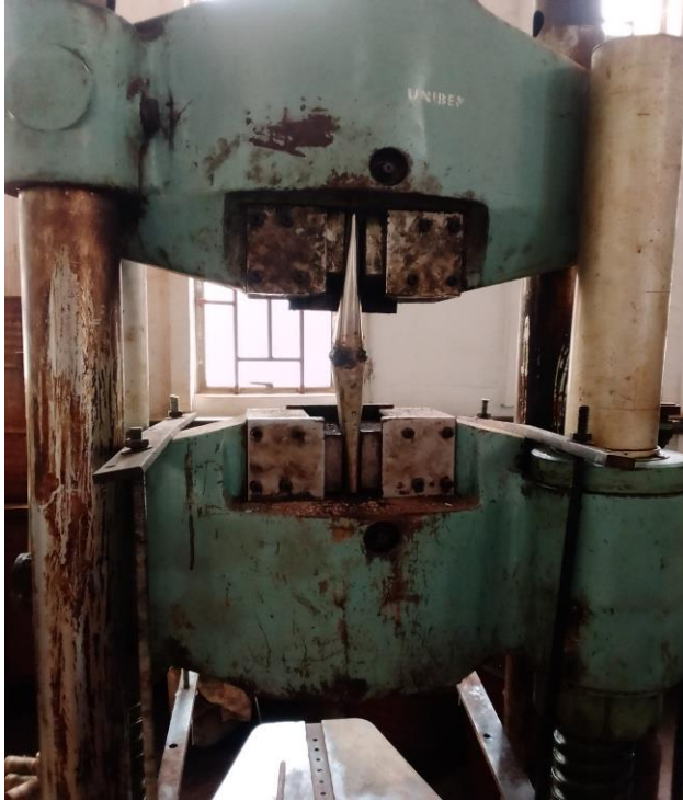
Fig 4.4(a): Specimen before Tensile Strength Test
