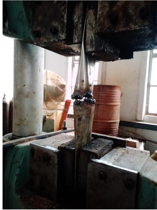
Fig 4.4(b): Specimen Failed after Tensile Strength Test
