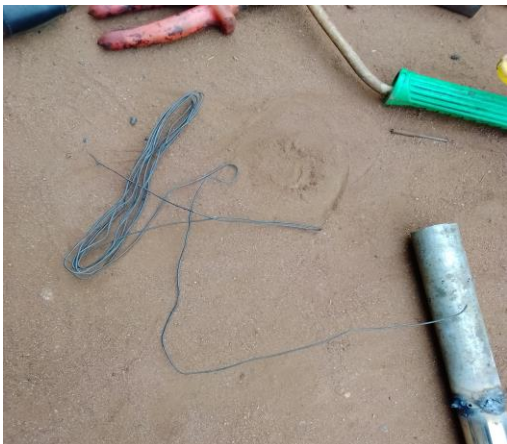
Fig 3.4: Binding wire used as filler in welding.
