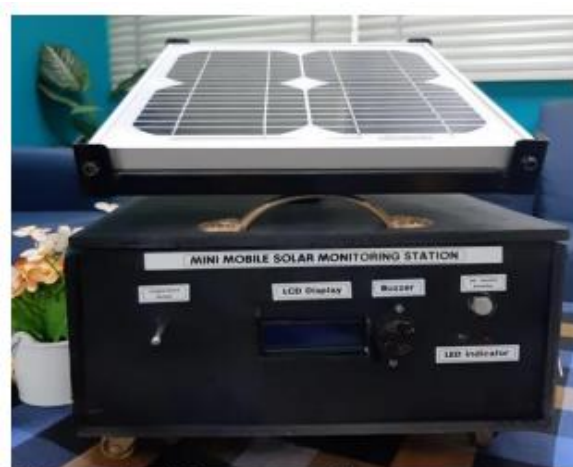
Figure 2. 17 Mobile Solar Power Monitoring Station Powered by IoT.
