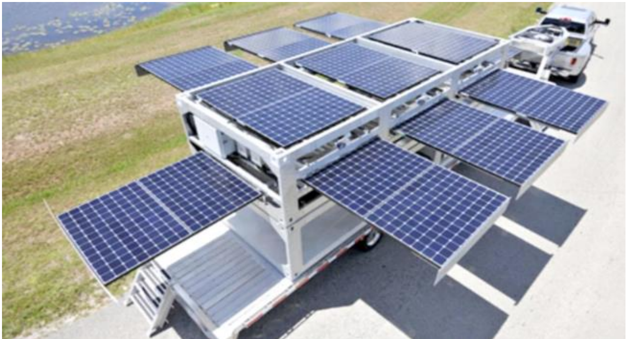
Figure 2. 18: Solar-powered portable electrical vehicle charging station.
