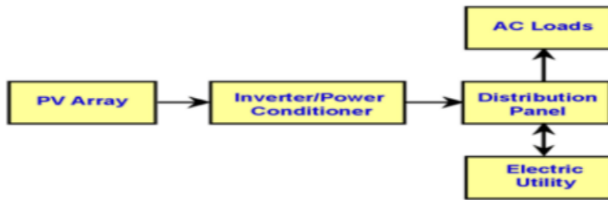
Figure 2. 1: Block Representation of Grid-connected solar system.
