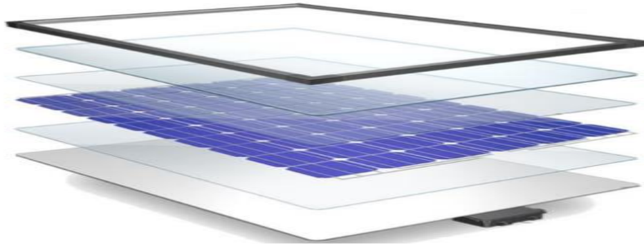
Figure 2. 5: P.V. module assembly
