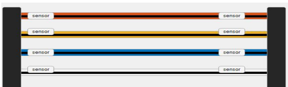
Figure 4.26: Three phase distribution line on MATLAB interface after restoration of broken yellow phase indicating all lines active.
