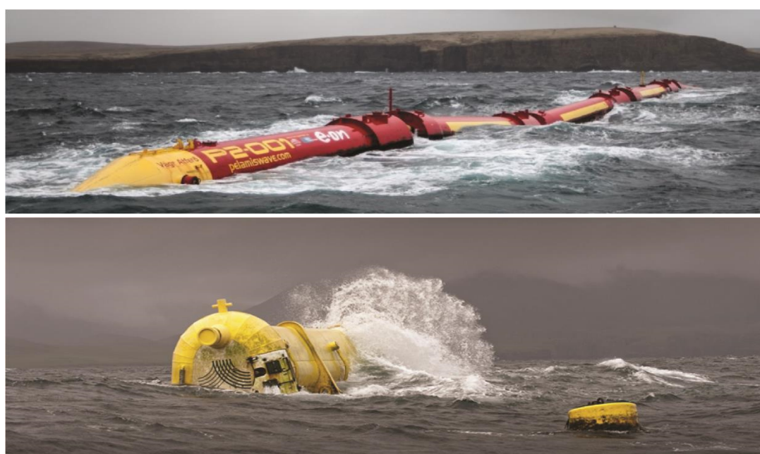
Figure 2.1 Pelamis P2-001 wave energy converter of Pelamis Wave energy during testing at the European Marine Energy Centre (EMEC) in Orkney, Scotland, in 2010.
