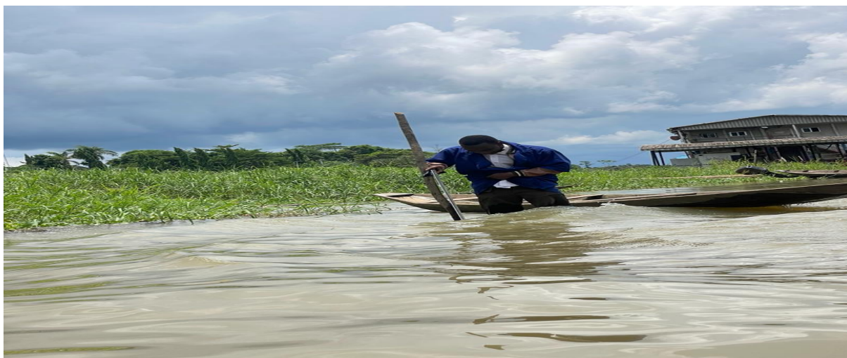
Figure 3.5 Photo of the fixed stick calibrated for measuring the wave height
