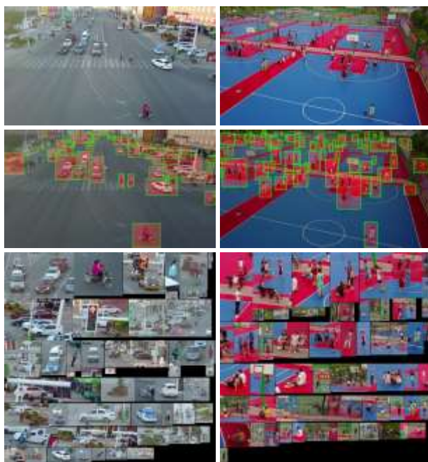
Figure 2.6: Visualization of UFP. Top: input images; middle: clustered regions highlighted by green bounding boxes; and bottom: packed mosaics.
