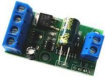
Fig 2.5: Voltage Converter Module
