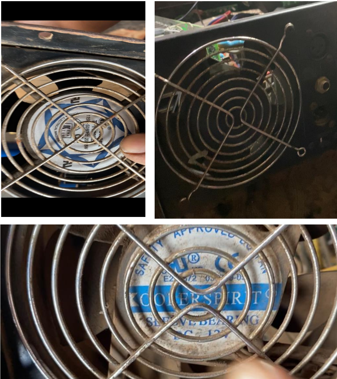
Figure 3.8: ac fan with ratings:220V 50/60Hz;80W
