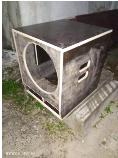
Figure 3.9: cabinet after cutting to size and applying adhesive.
