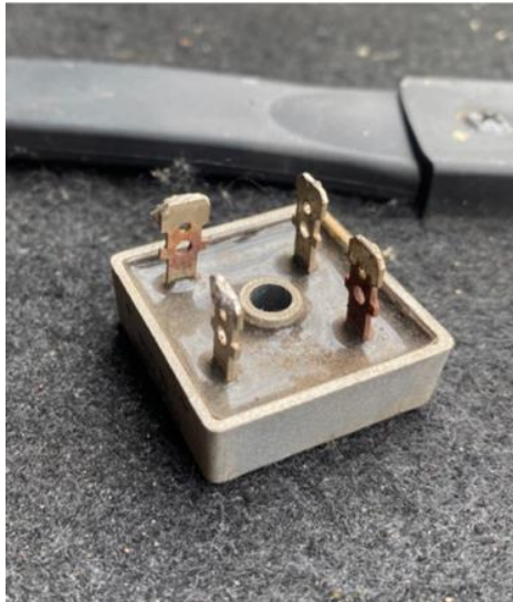
Figure 2.17: A 50Amp bridge diode rectifier
