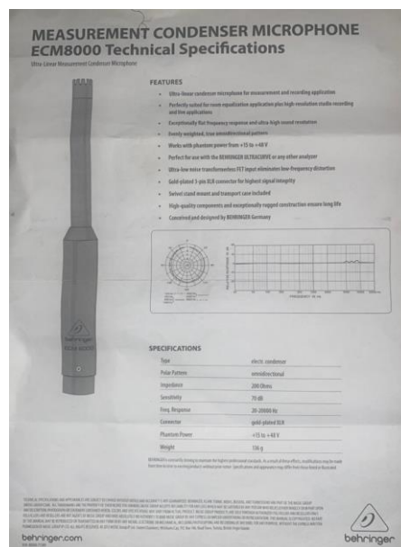
Figure 3.14: the specification sheet showing the frequency response of the measurement microphone and the polar response respectively.
