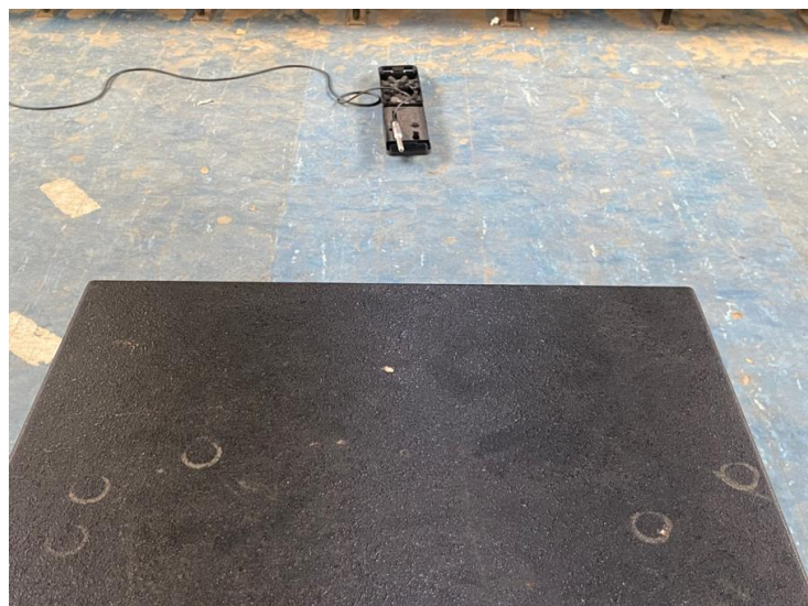
Figure 4.3: microphone position in front of device under test.
