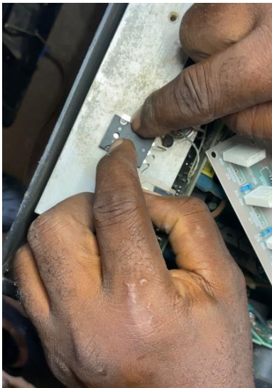
Figure 3.7: an aluminum heat sink used for the dissipation of heat from the transistors (22 x10x2.5 centimeters)
