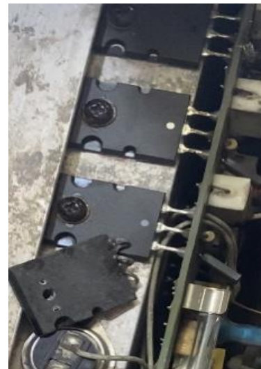
Figure 3.7: an aluminum heat sink used for the dissipation of heat from the transistors (22 x10x2.5 centimeters)
