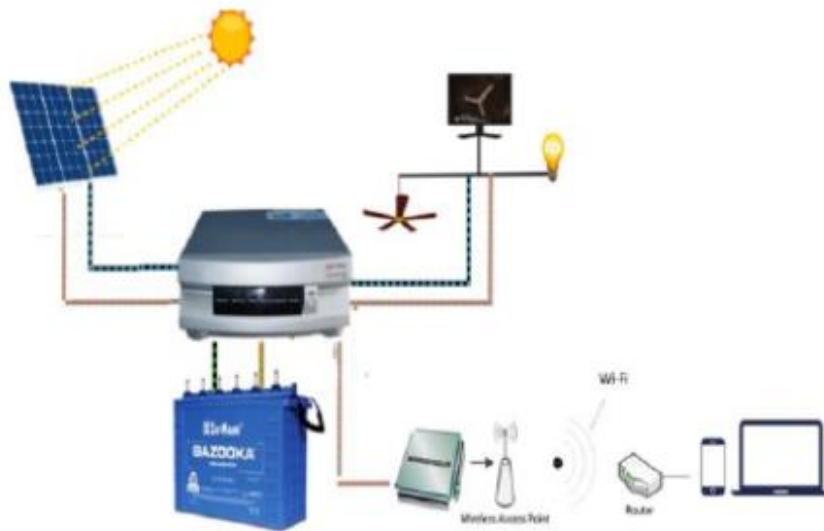
Figure 1: Functional Architecture of the Proposed IoT-Based Smart Controlled Inverter
