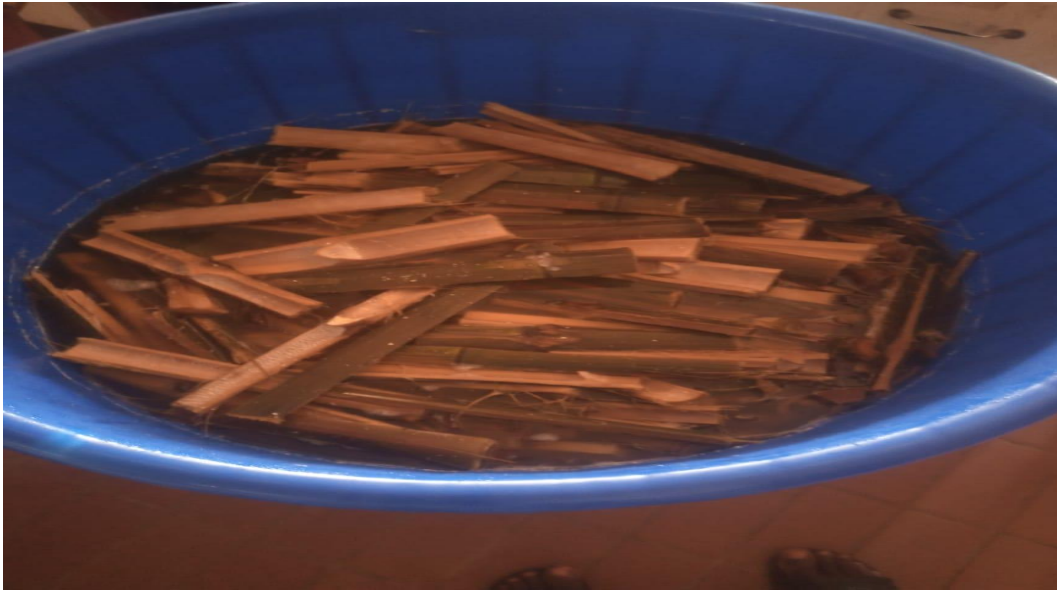
Plate 3.2 Bamboo Soaked in Delignification Bath
