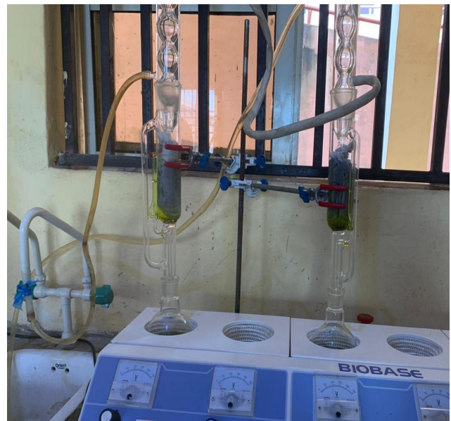
Plate 3: Showing the process of extraction of ocimum gratissimum using soxhlex extractor. Photocredit: (Ani Victoria, 2025).
