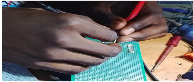
Fig 4.5: Carrying out a continuity test using multimeter in order to check for any bridge in the main circuit before mounting the ESP32 Dev module
