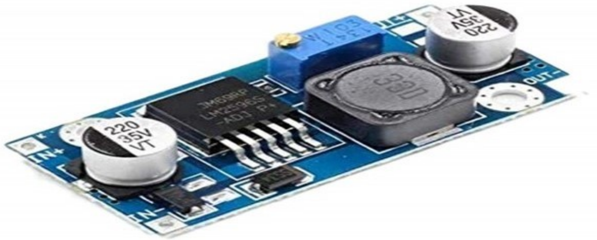
Fig 2.6: LM-2956 DC-DC Bulk Converter
