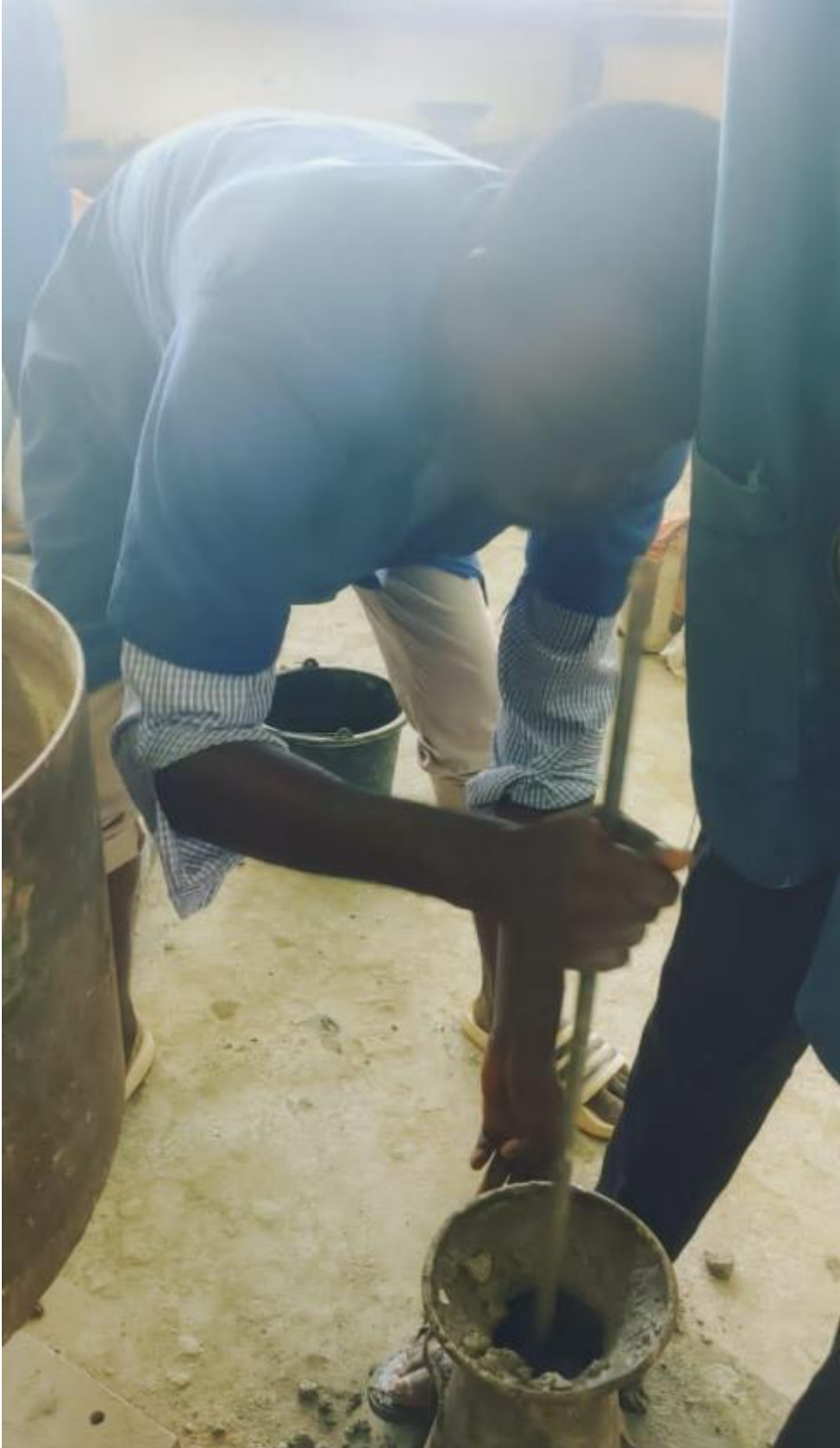
Plate D3: Tamping the concrete in the slump cone
