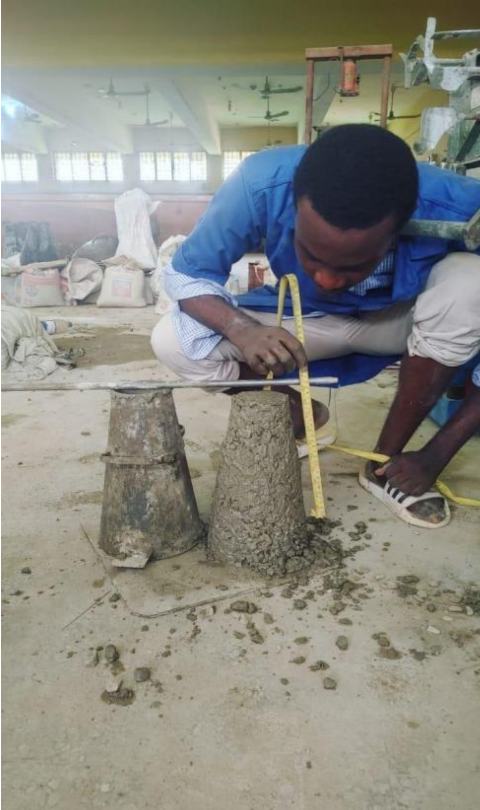
Plate D2: Performing the slump test to determine the workability of fresh concrete
