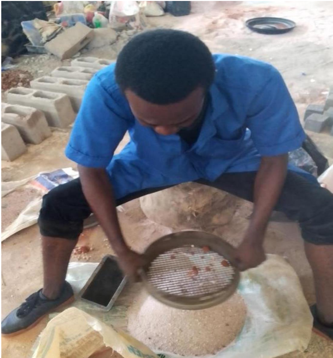
Plate D1: Sieving of fine aggregate (sand) during sample preparation
