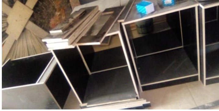
Plate 7: Title: Application of HDF Edge Tapes on the HDF Boards Source; Textile Studio Year: 2021
