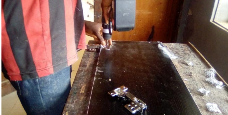
Plate 5: Title: Joining of HDF Boards Source; Textile Studio Year: 2021
