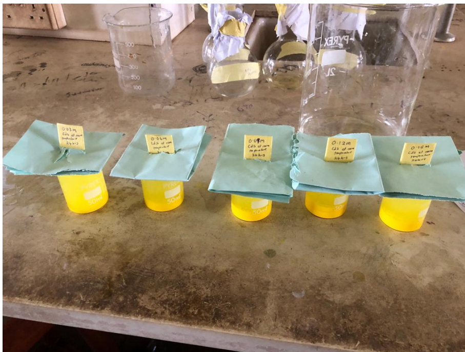
Figure 3. 2 Thin films deposited in Strontium Iodide with molar concentration of 0.12 mol/dm 3 and at room temperature.
