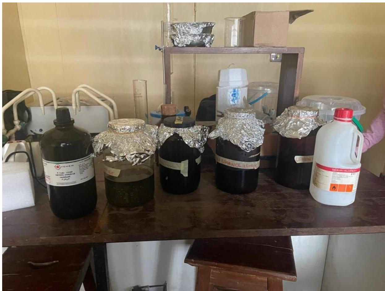
Extraction using ethanol (polar) and diethyl ether (non-polar) in brown glass jars
