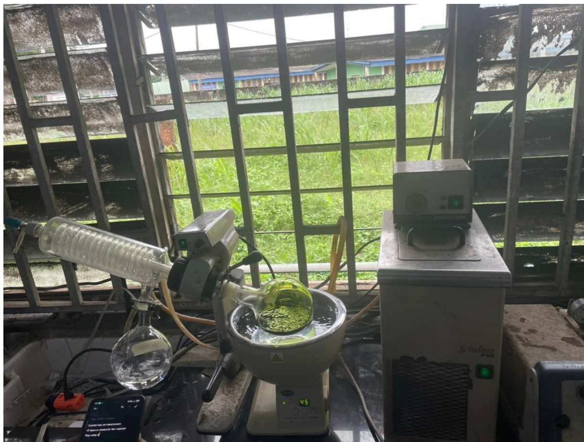
Concentration and solvent extraction using Rotary evaporator
