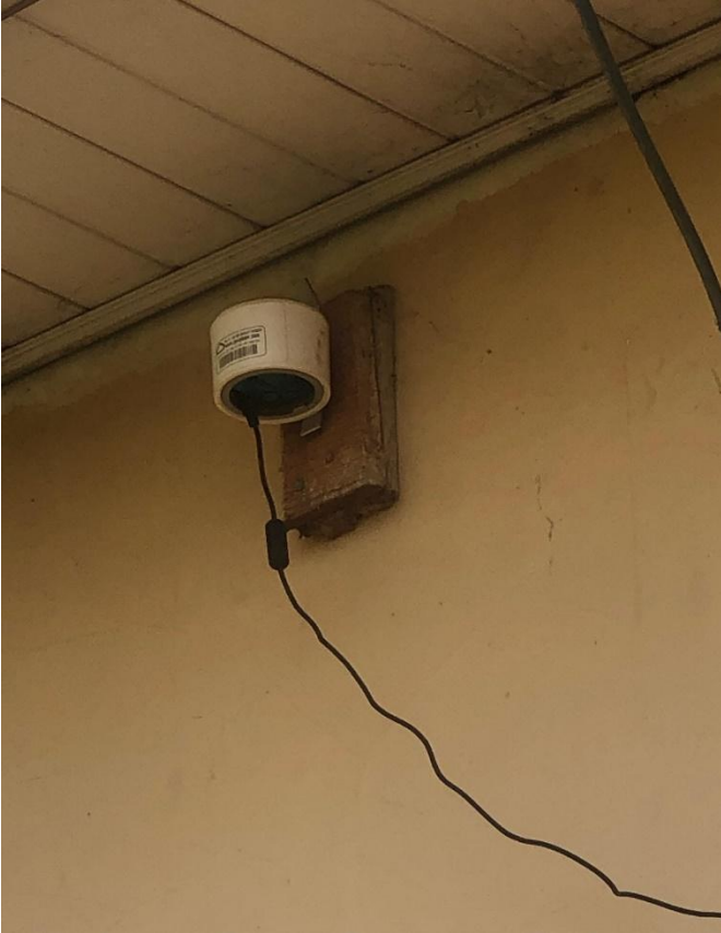
PurpleAir Sensor Installed in University of Benin (UNIBEN)
