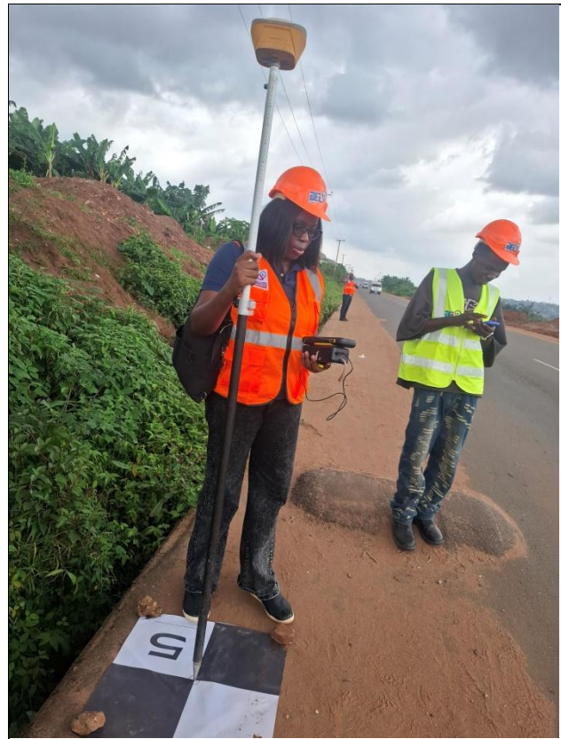
Fig 3.4d Captured accurate geographical coordinates of a GCP marked on ground
