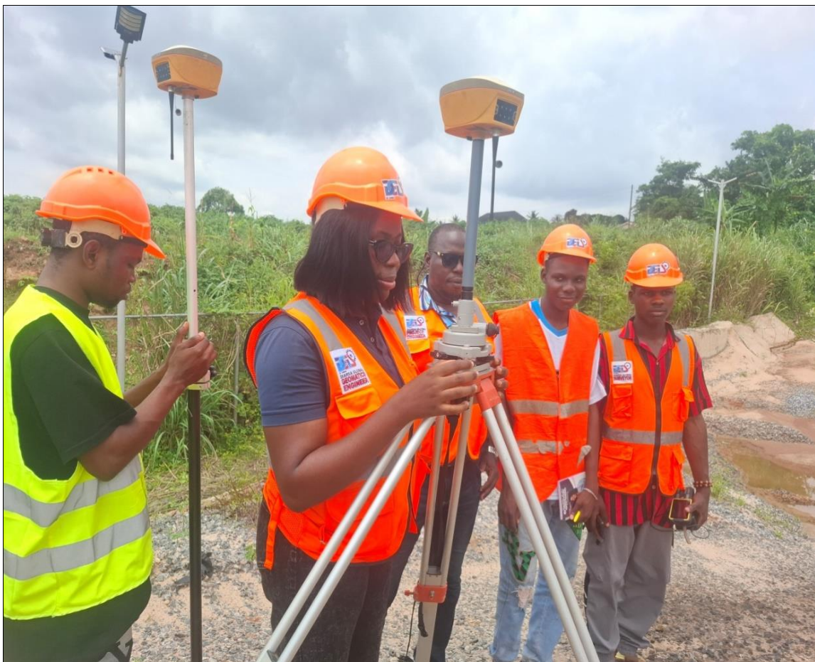
Figure 3.4a: GNSS Base and Rover set up at Temboga site
