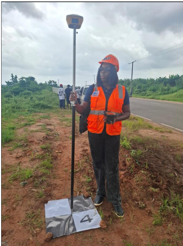
Fig 3.4d Captured accurate geographical coordinates of a GCP marked on ground
