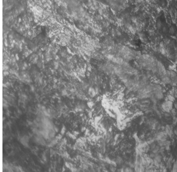
Plate A.1q: Optical Micrograph of the Heat Affected Zone (HAZ) of 0.36%C Steel annealed at 920 °C for 3hr 30min at X1000.
