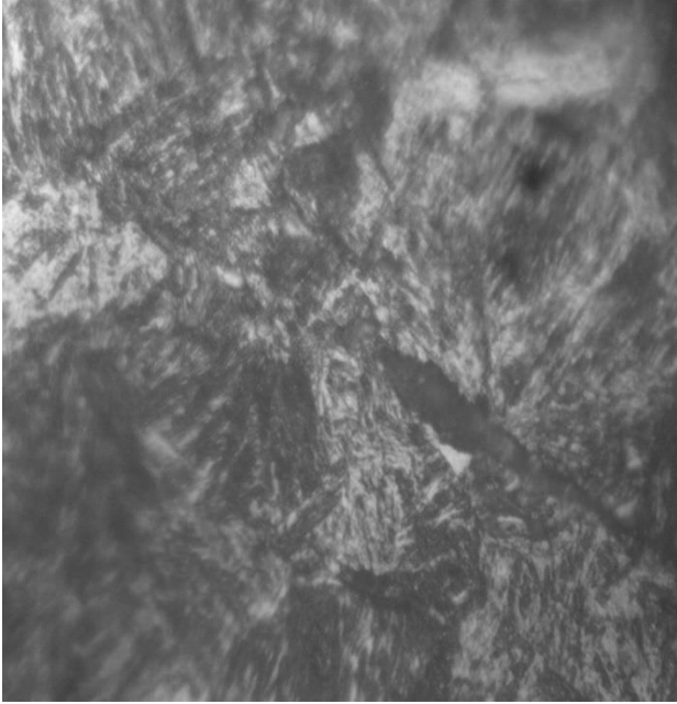
Plate 4.1m: Optical Micrograph of the Parent Metal of 0.36%C Steel annealed at 860 °C for 2hr 30min at X1000. Structure shows packet and block martensite lath with very little patches of retained austenite grains.
