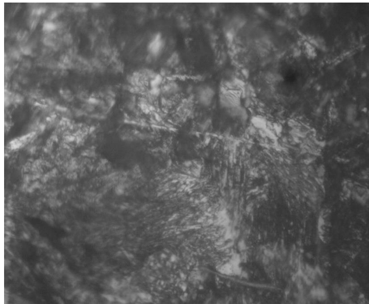
Plate A.1r: Optical Micrograph of the Welded Zone of 0.36%C Steel annealed at 1000 °C for 3hr 30min at X1000
