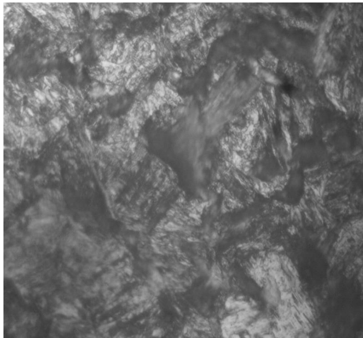
Plate 4.1u: Optical Micrograph of the Welded Zone of 0.36%C Steel annealed at 860 °C for 3hr 30min at X1000. Structure shows packet and block of martensite lath with traces of retained austenite.
