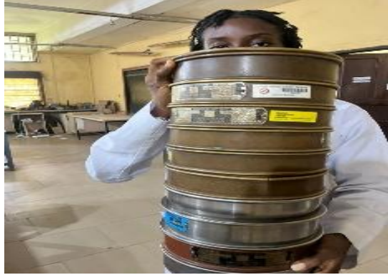
Plate D: High Precision Test Sieves (ASTM Standard)
