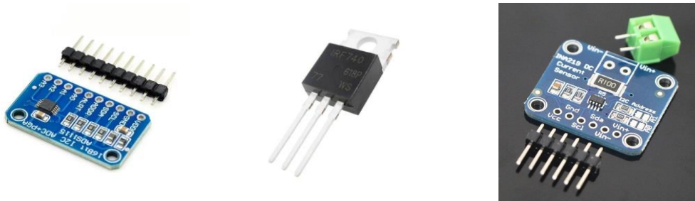
Figure 3.4: ADS1115 ADC Module, IRLZ44N N-MOSFET, INA3221 Voltage/Current Sensor
